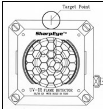
Figure 14: UV/IR Detector Target Point
